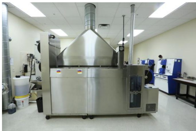
Kofile's microfilm processor (center) and duplication machine (far right).
